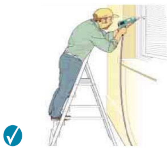
Correct – steps facing work activity
