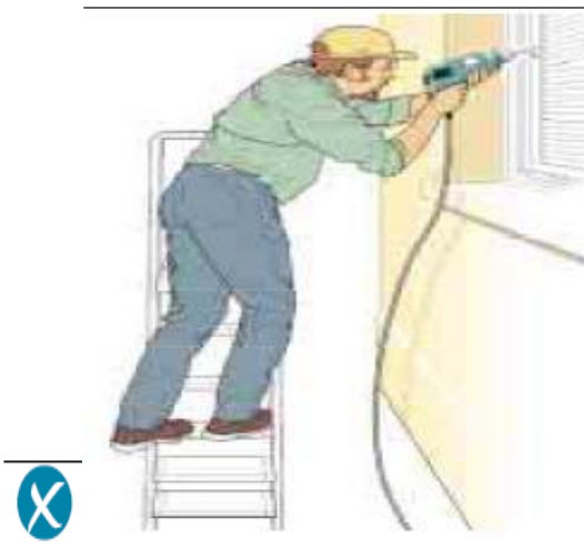
Incorrect – steps side on to work activity
